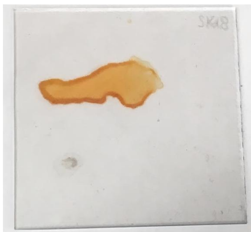
Figure 7: Photographic Sample of SK-18. The plate contains a 300 \mu\text{L} spot of 0.05 M \text{Fe}(\text{NO}_3)_3 with 1% \text{La}(\text{NO}_3)_3 , and a 5 \mu\text{L} spot of 0.05 M \text{Cu}(\text{NO}_3)_2 .
