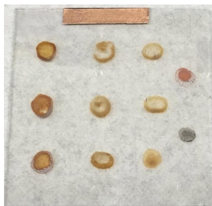
Figure 5: Photographic Sample of SK-17. The first column features 20 \mu\text{L} spots at a 4:1:1 volume ratio of 0.05 M \text{Fe}(\text{NO}_3)_3 to 0.05 M \text{Ni}(\text{NO}_3)_2 to 0.05 M \text{Zn}(\text{NO}_3)_2 . The second column features 20 \mu\text{L} spots at a 1:4:1 volume ratio of 0.05 M \text{Fe}(\text{NO}_3)_3 to 0.05 M \text{Ni}(\text{NO}_3)_2 to 0.05 M \text{Zn}(\text{NO}_3)_2 . The third column features 20 \mu\text{L} spots at a 1:1:4 volume ratio of 0.05 M \text{Fe}(\text{NO}_3)_3 to 0.05 M \text{Ni}(\text{NO}_3)_2 to 0.05 M \text{Zn}(\text{NO}_3)_2 . In the last column, 0.05 M \text{Fe}(\text{NO}_3)_3 was spotted on top and 0.05 M \text{Cu}(\text{NO}_3)_2 was spotted below at 20 \mu\text{L} as well, to function as standards.
