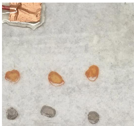
Figure 2: Photographic Sample of SK-11. The top row contains 10 \mu\text{L} spots of 0.05 M \text{Fe}(\text{NO}_3)_3 . The bottom row contains 10 \mu\text{L} spots of 0.05 M \text{Cu}(\text{NO}_3)_2 .
