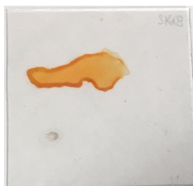
Figure 9: Plate SK-18; includes one big spot of 99% iron(III) nitrate and 1% lanthanum(III) nitrate, and a faint spot of copper that was picked up in scans at the beginning.
