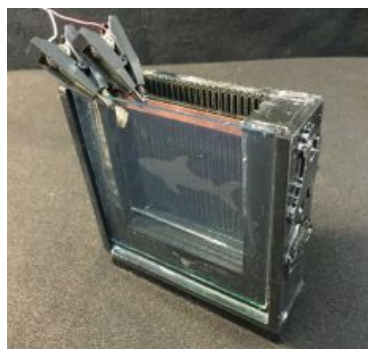
Figure 3: Alligator clips attached to kit (white wire--black wire in the kit used for this experiment--is attached to the FTO glass cover of holder, while red wire is attached to copper tape on FTO sample glass plate).
