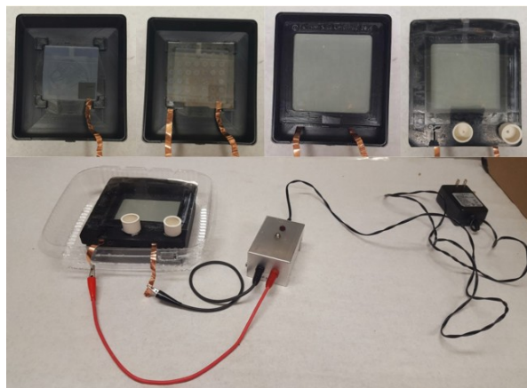
Figure 8. Top (from left to right): 3-D printed holder with FTO plate counter-electrode; FTO plate spotted with metal oxides; mesh secured by mesh holder; holder lid with window and septa. Bottom: Full 3-D printed holder setup.
