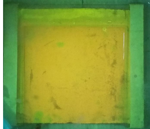
Figure 6. Results from running a 0.05M MnO 2 plate in 0.1M H 2 SO 4 (pH 2.5).
