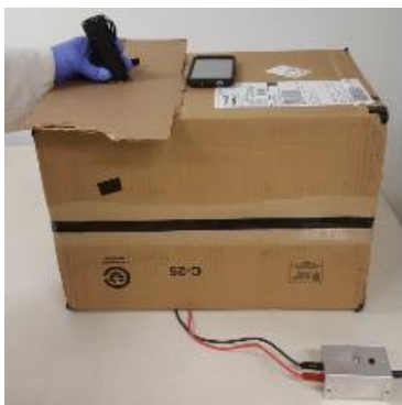
Figure 4. Box used for 3D-printed holder had a hole on top for flashlight and a hole next to it for the filter.
