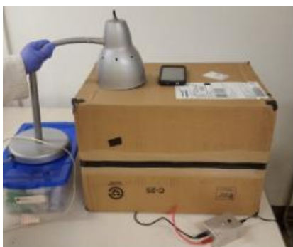
Figure 5. A bigger hole was made on the top of the box for the 3D-printed holder to fit the rim of the lamp.
