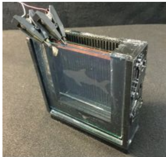
Figure 4: The 3-D printed sample well.
