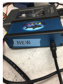
Figure 5: The new electronics box after being attached to MyRIO
