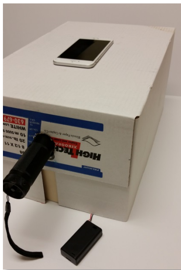
Figure 9: Box with camera phone, LED flashlight, and power supply positioned for data collection.
