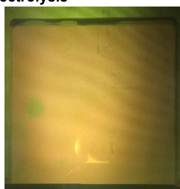
Figure 10B. Illuminated electrode appears orange and is ready for electrolysis
