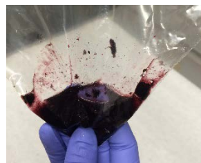
Figure 13. A crushed berry releases juice that we can use to dye our TiO 2 slide.
