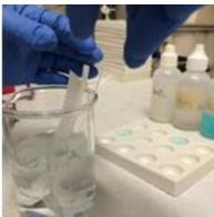
4. Select two metals to be tested (see student data table below), and place one end of the salt bridge in the well of one metal, and the other end of the salt bridge in the well of the other metal. Be sure that each end is touching the solution. Tweezers can help for this step but are not necessary as the NaCl solution is harmless. One person in the group will need to hold the bridge there as a teammate completes the next steps.
